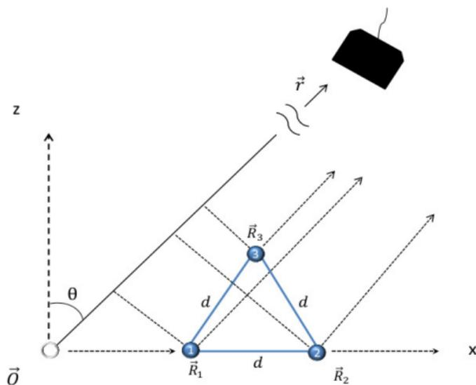
**Figure:** Schematic diagram of the system: where three identical and equidistant two-level atoms are localized at the vertices of an equilateral triangle. A detector at position  $\vec{r}$  records the photon scattered by the atoms, in the far field regime.
