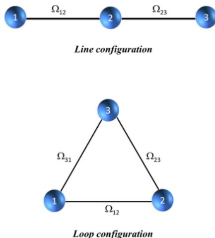
**Figure:** Schematic representation of Line(open loop) and Loop (closed loop) configurations for three qubits coupled via dipole-dipole interaction.
