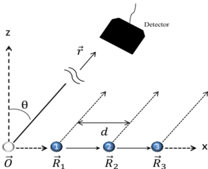
**Figure:** Schematic diagram of the system: where three identical two-level atoms are localized at positions  $\vec{R}_1$  to  $\vec{R}_3$ . A detector at position  $\vec{r}$  records a photon scattered by the atoms, in the far field regime.
