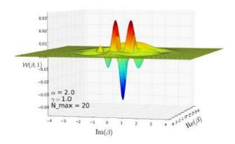
Wigner function  $\mathcal{W}(\beta,\gamma)$  of the post-measurement state of  $|\psi_{\alpha}\rangle$  after sharp measurement with  $O^4(\frac{\pi}{4})\otimes O^4(\frac{3\pi}{4})$ , N\_max is the maximum number of photons in each mode
