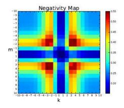
Wigner function negativity of the post-measurement state of  $|\psi_{\alpha}\rangle$  after sharp measurement with  $O^{k}(\frac{\pi}{4}) \otimes O^{m}(\frac{3\pi}{4})$ for different values of k and  $m \cdot \mathcal{N}_{\psi}$  has  $\ell m - \nu e$ Value for k = m = 0 compared to other Values of k and  $m \cdot$
