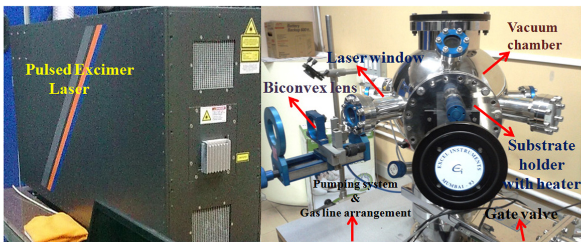
Figure 2.4 PLD setup in our lab. Courtesy: Ref. [82].
