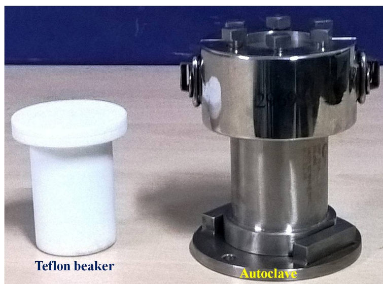
Figure 2.2 Image of Autoclave with Teflon beaker.
