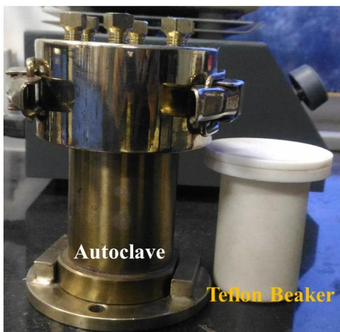
*Figure 2.7: Autoclave with Teflon beaker*
