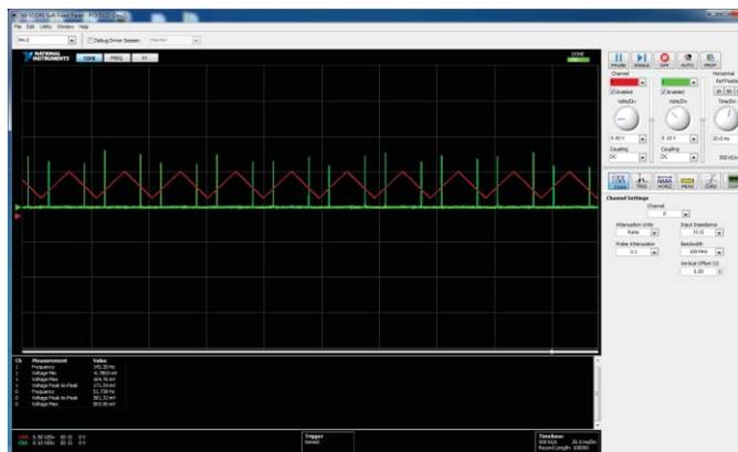
**Figure 4.4** Screen shot of National instrument scope in the desktop of data acquisition PC during the experiment. The red coloured triangular voltage periodically modulates the cavity length and the subsequently green coloured spike is appeared due to generating intracavity light for mode matching inside the cavity.
