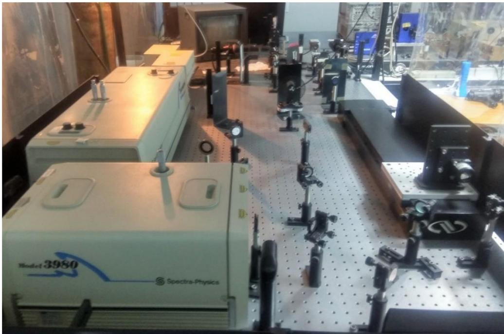
**Figure 3.12** Photograph of the collinear TR-MOKE setup at S. N. Bose National Centre for Basic Sciences.
