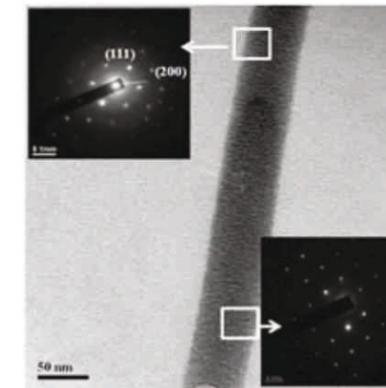
Fig.1: High resolution transmission electron micrograph of a cobalt nanofiber prepared by an electrospinning technique. Selected area diffraction (inset) shows large uniformity of the sample.
