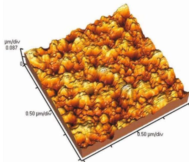
Fig. 1: AFM of CoNiAl alloy – thin film (3-D)
