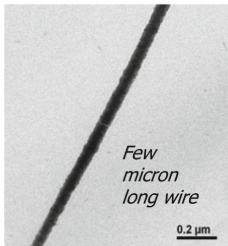
Fig.1: A 35nm Single Crystalline Ni Nanowire grown by electro deposition.
