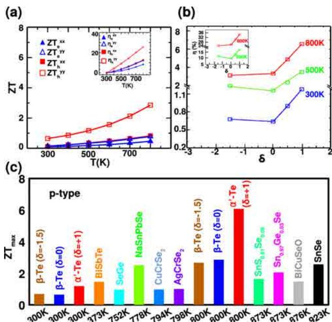
**Figure 2:** (a) The temperature variation of ZT and TE efficiency (inset) of unstrained Te monolayer, for chosen carrier concentration of  $10^{13} \text{cm}^{-2}$ . (b) The variation of ZT with strain at  $T=300$  K,  $500$  K, and  $800$  K. The inset shows the corresponding variation of TE efficiency at  $500$  K and  $800$  K. (c) Comparison of TE performance of strained and unstrained Te monolayer with other known p-type layered materials.
