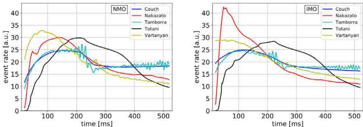
**Figure 2:** Expected event rates at Hyper-Kamiokande experiment for different core-collapse models for two mass hierarchies, normal (left) and inverted (right).
