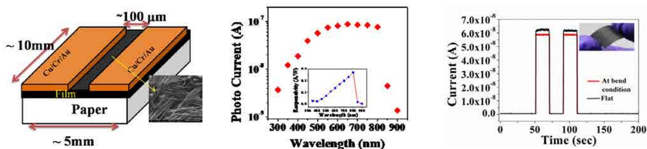
3.(a) Schematic of the wearable electronics based flexible photo detector, (b) Spectral Response of the photo current (illumination intensity  $120 \mu\text{W}/\text{cm}^2$ ) Inset: Spectral dependence of the Responsivity. (C) Comparison of response of flexible photo detector in flat/bend condition
