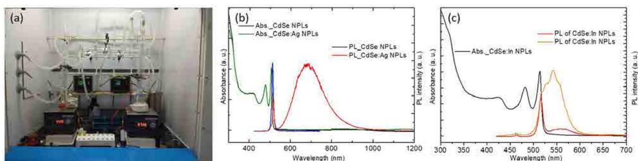
**Figure 1** (a) Picture of the newly assembled Schlenk line setup for the synthesis of colloidal nanocrystals. (b) Absorption and PL spectra of CdSe NPLs and CdSe:Ag NPLs respectively. (c) Absorption and PL spectra of CdSe:In NPLs.
