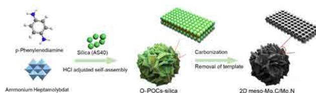
**Figure 1.** Scheme of synthesis of two-dimensional (2D) Mo-based carbides/nitrides.
